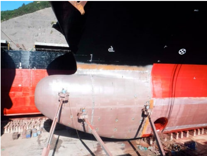
Optimised bulbous bow – M/V Ruby Tower
